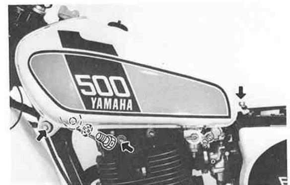
3. Remove the three bolts securing the fuel tank the frame and remove the fuel tank.
