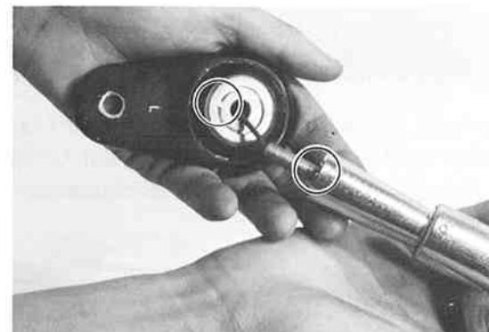
4. Fit the flasher light lead wire with the special washer (n-8), negative lead wire (n-11), spring washer (n-9) and nut (n-10) in this order; then tighten the nut.
